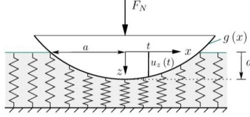
**Fig. 4** Equivalent model for a Hertzian contact
