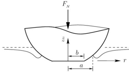
**Fig. 6** Qualitative presentation of the adhesive contact of a parabolic profile with a flattened tip
